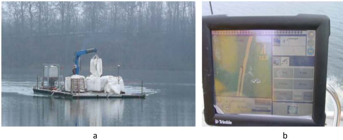
Figure 7. Large application system with coupled pontoons and crane installed on board (a), GPS system (b)
