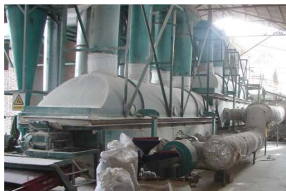
Figure 2. Phoslock manufacture at the Phoslock® manufacturing factory (a), Dewatering and drying processes during the Phoslock® manufacturing (b).
