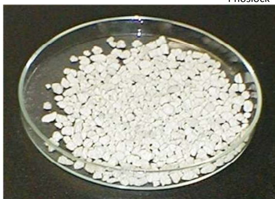
Figure 3. Dry, free flowing granular Phoslock® (0.5 – 3 mm) and packet format: 25 kg Phoslock® bags.
