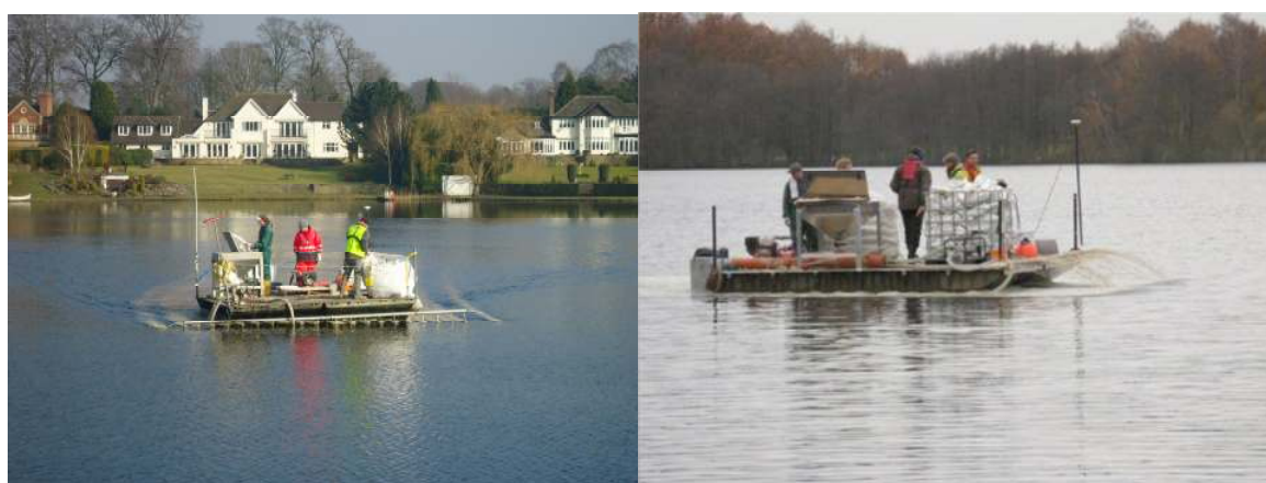
Figure 6. Application of Phoslock®; pontoons with mounted mixing and application system
